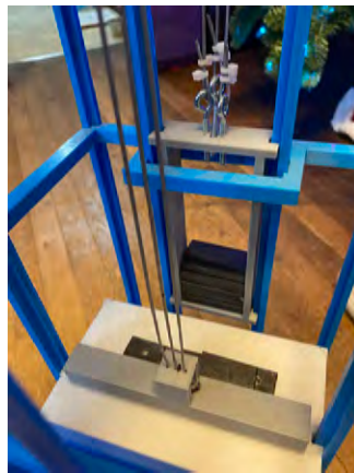
Hoistway cables attached to the car top and counterweight
