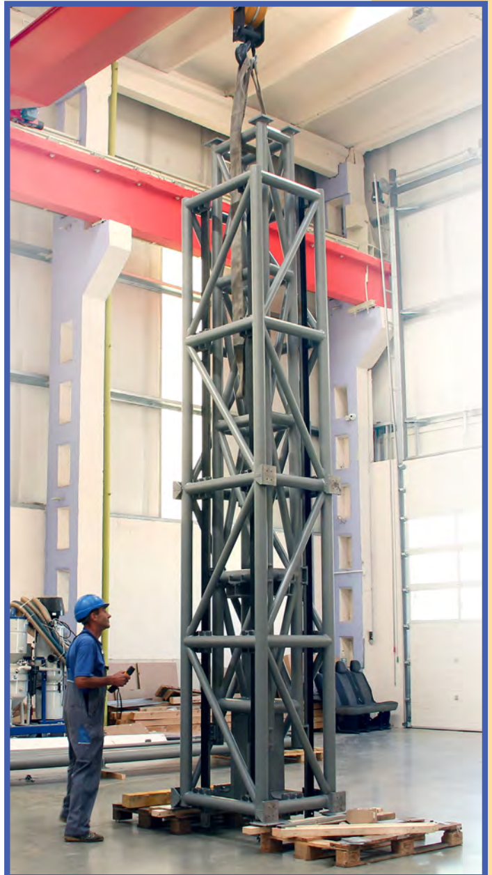
Drive system pre-assembling phase
