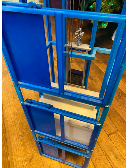
The hoistway of the model elevator: the blue panels are the hall doors.
